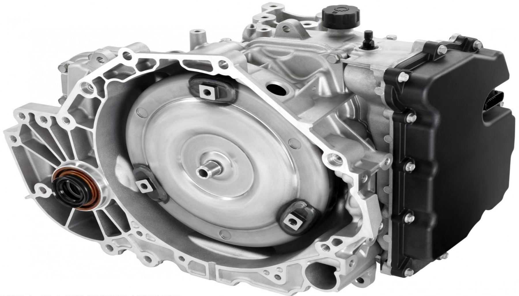
2011 Hydra-Matic 6T45 (MH7) FWD / (MHC) AWD Six Speed Automatic Transaxle
