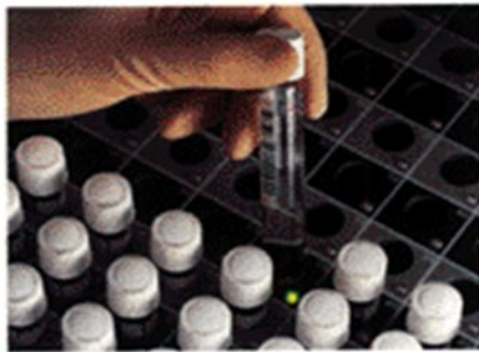
Step 3: Load where indicated by green LED.
