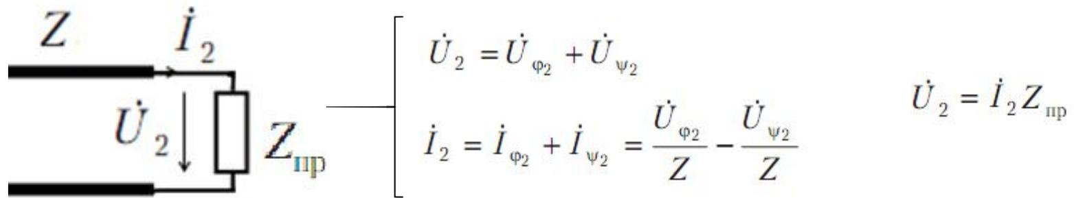
$$2\dot{U}_{\psi_2} = \dot{U}_2 - \dot{I}_2 Z = \dot{I}_2 (Z_{\text{нр}} - Z); \quad 2\dot{U}_{\varphi_2} = \dot{U}_2 + \dot{I}_2 Z = \dot{I}_2 (Z_{\text{нр}} + Z)$$
