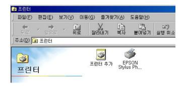
After selecting the tab in detail in the registered information, confirmEPUSBx:(EPSON STYLUS PHOTO 1290 or 890) is displayed in the port list to be printed. For Windows 2000 User, press the port tab, and confirm ifUSBxxx,EPSON STYLUS PHOTO 1290 or 890 is displayed in the port list to be printed.
