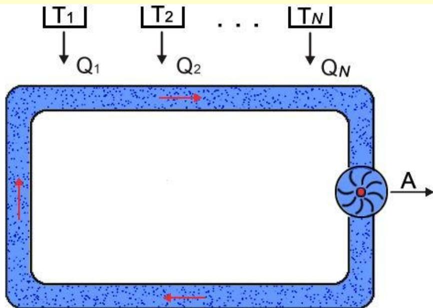
$$\frac{Q_1}{T_1} + \frac{Q_2}{T_2} + \dots + \frac{Q_N}{T_N} \leq 0$$
