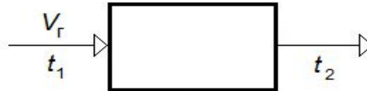
$$P(Q_{\text{тех}} + Q_{\text{o.c}}) = V_{\Gamma} c_{\Gamma} (t_1 - t_2), \quad \Delta t = t_1 - t_2 \quad \uparrow V_{\Gamma} \Rightarrow \downarrow \Delta t$$
