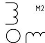
Microphone: 1-2. Common. 3. Condenser. 4. Piezoelectric.
