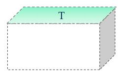
Temperature at the boundary of the body is given as a function of time and position or simply as a constant value
