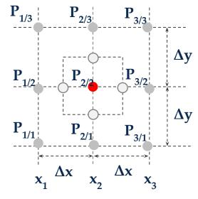
$$\frac{\partial \theta}{\partial x}\Big|_{P2/2} \approx \frac{\frac{\partial \theta}{\partial x}\Big|_{P1.5/2} - \frac{\partial \theta}{\partial x}\Big|_{P2.5/2}}{dx} = \frac{\left(\frac{\theta_{2/2} - \theta_{1/2}}{dx}\right) - \left(\frac{\theta_{3/2} - \theta_{2/2}}{dx}\right)}{dx} = \frac{2 \cdot \theta_{2/2} - \theta_{1/2} - \theta_{3/2}}{dx^2}$$
