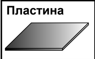
$$M_x = D \left( \frac{\partial^2 w}{\partial x^2} + \mu \frac{\partial^2 w}{\partial y^2} \right)$$
