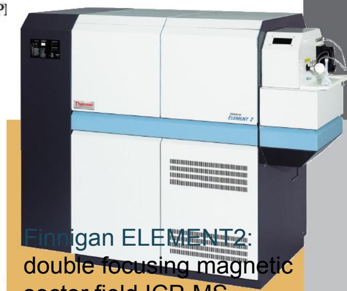
Finnigan ELEMENT 2: double focusing magnetic sector field ICP-MS.
