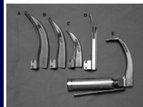
Figure 3. Lateral view of straight and curved laryngoscope blades. A–C, Mackintosh Blades (sizes 4, 3, and 2). D, Miller blade; E, McCoy blade (tip in “elevated” position).
