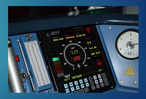
This is how the modern cab of an electric locomotive driver looks like. Here is a modern model of the TFT Module in the rolling stock of railway transport.
