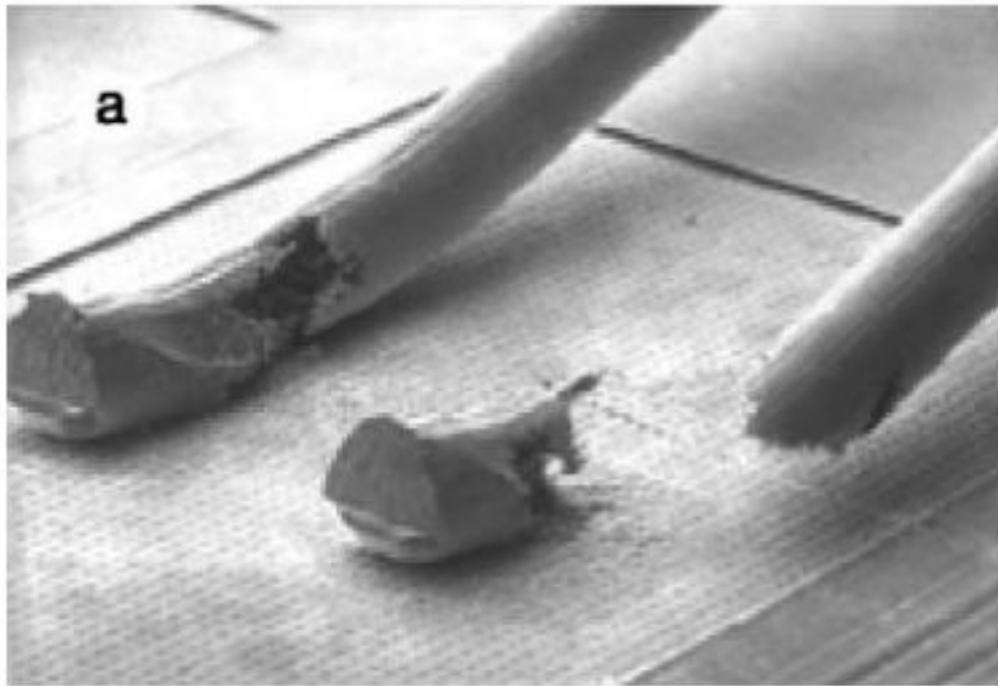
Fig. 15. (a) Rupture of emitter bond wires due to stress corrosion (SEM image, 30 \times ). (b) Detail of a corroded emitter bond wire (SEM image, 80 \times ).
