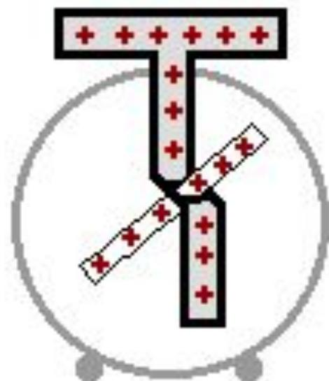
**Grounding a positively-charged electroscope involves the transfer of electrons from "the ground" to the electroscope.**
