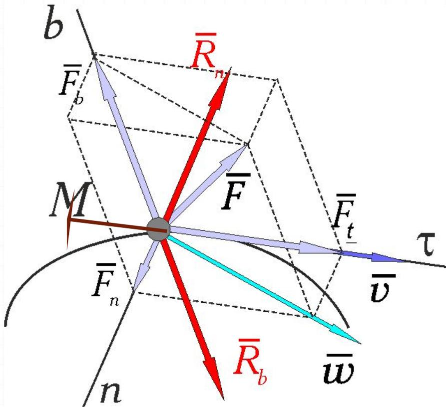
$$\left\{ \begin{array}{l} \ddot{ms} = F_{\tau} (t, \dot{s}, s); \\ m \frac{\dot{s}^2}{\rho} = F_n + R_n; \quad F_{\tau \rho}; \\ m \frac{\rho \dot{s}^2}{\rho} = F_b + R_b; \quad R_n; \\ 0 = F_b + R_b. \end{array} \right.$$
