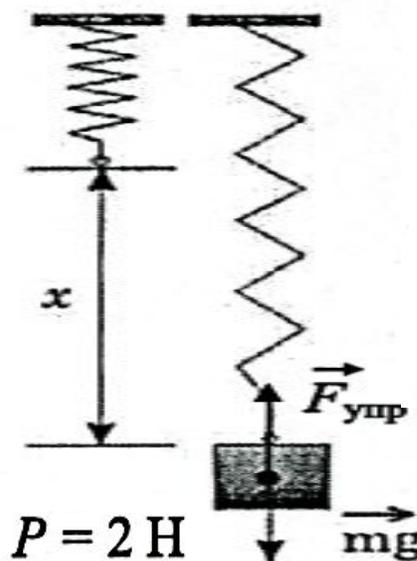
$$2) F_{\text{упр}} = mg = P; F_{\text{упр}} = kx; \Rightarrow k = \frac{P}{x};$$
