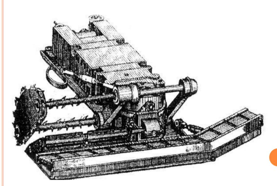
This was the first machine that performed notching, chipping and piling coal simultaneously.
