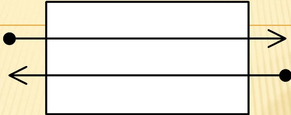
$$\left\{ \begin{array}{l} \frac{dT_1}{d\tau} + a \frac{dT_1}{dx} = b_1 (T_{\text{CT}} - T_1) \\ \frac{dT_{\text{CT}}}{d\tau} = \beta_1 (T_1 - T_{\text{CT}}) + \beta_2 (T_2 - T_{\text{CT}}) \\ \frac{dT_2}{d\tau} - a_2 \frac{dT_2}{dx} = b_2 (T_{\text{CT}} - T_2) \end{array} \right.$$
