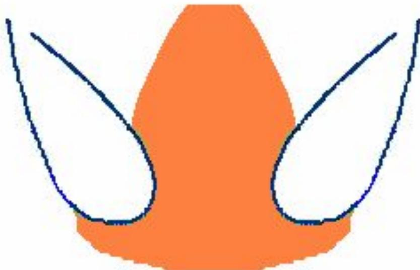
$$x_{\min} = \frac{h_a^* \cdot (z_{\min} - z)}{z_{\min}}$$
