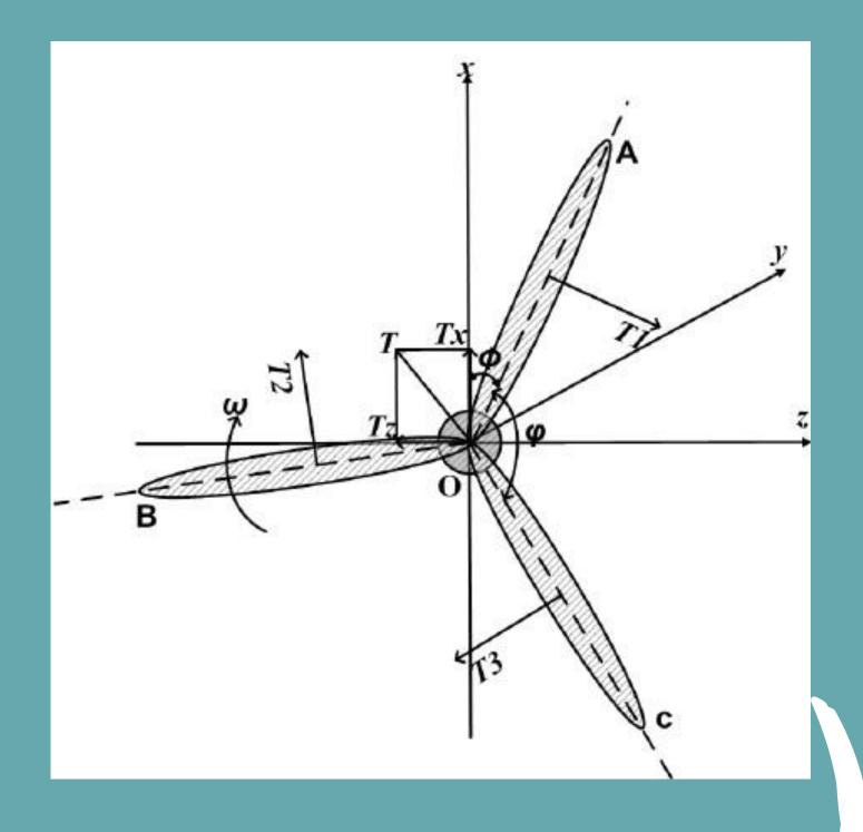
The swept area of the turbine can be calculated from the length of the turbine blades using the equation for the area of a circle:
