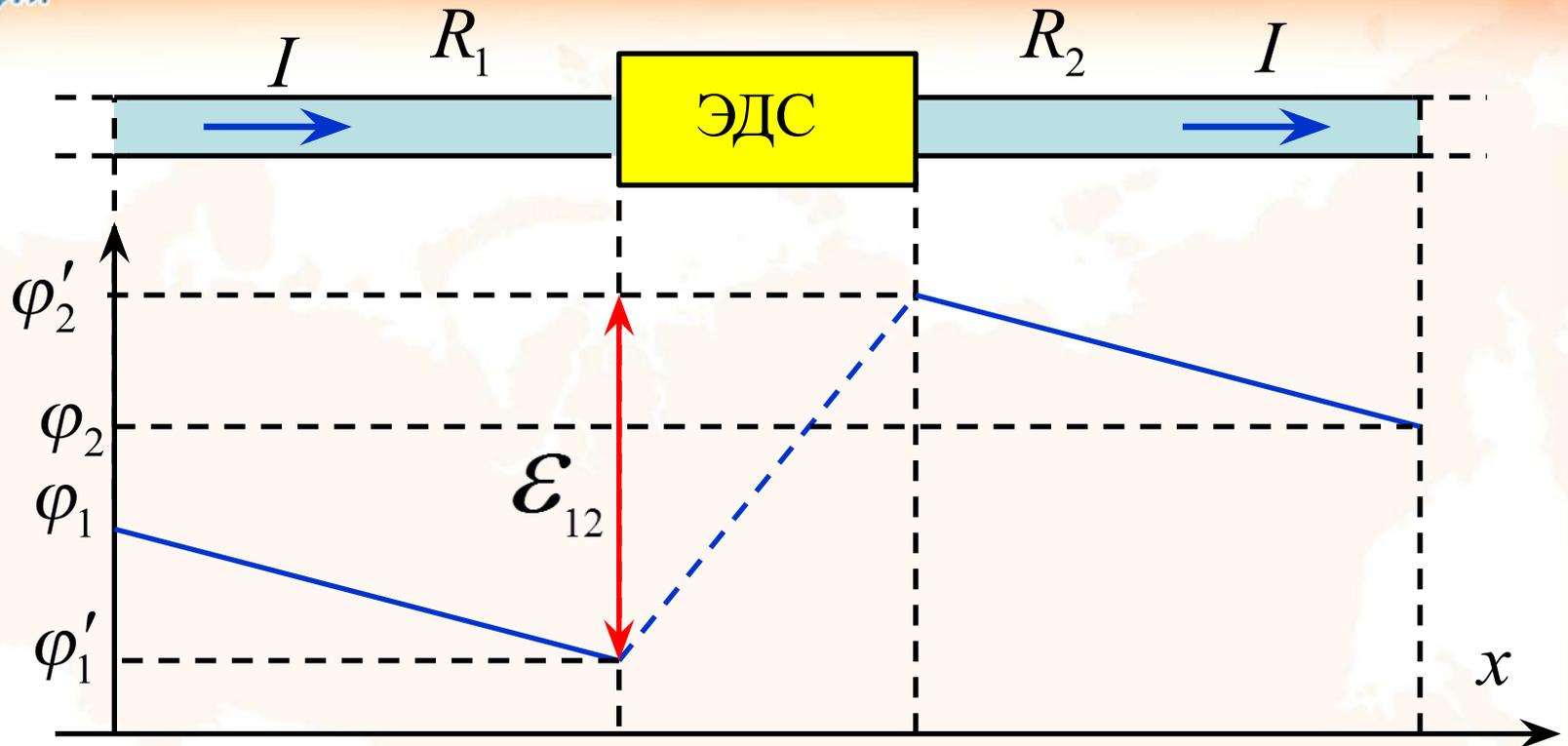
$$\begin{cases} IR_1 = \varphi_1 - \varphi_1' \\ IR_2 = \varphi_2' - \varphi_2 \end{cases} + I(R_1 + R_2) = \varphi_1 - \varphi_2 + \varphi_2' - \varphi_1' \Rightarrow$$
