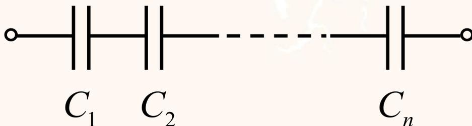
$$\frac{1}{C_{\text{общ}}} = \frac{1}{C_1} + \frac{1}{C_2} + \dots + \frac{1}{C_n}$$
