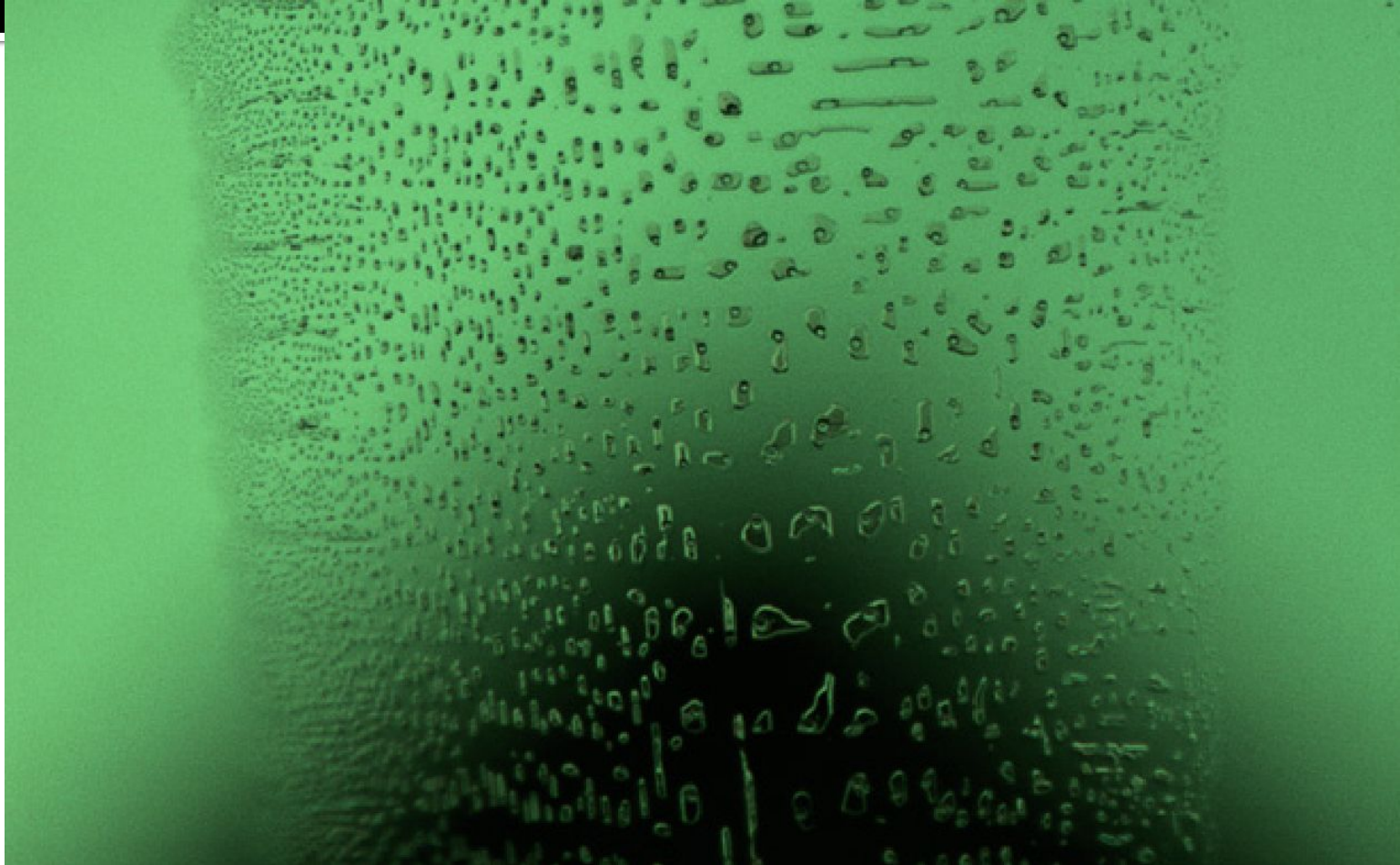
Flux residue often contains a contraction bubble, as seen in each of these trapped flux droplets. Field of view 1.08 mm
