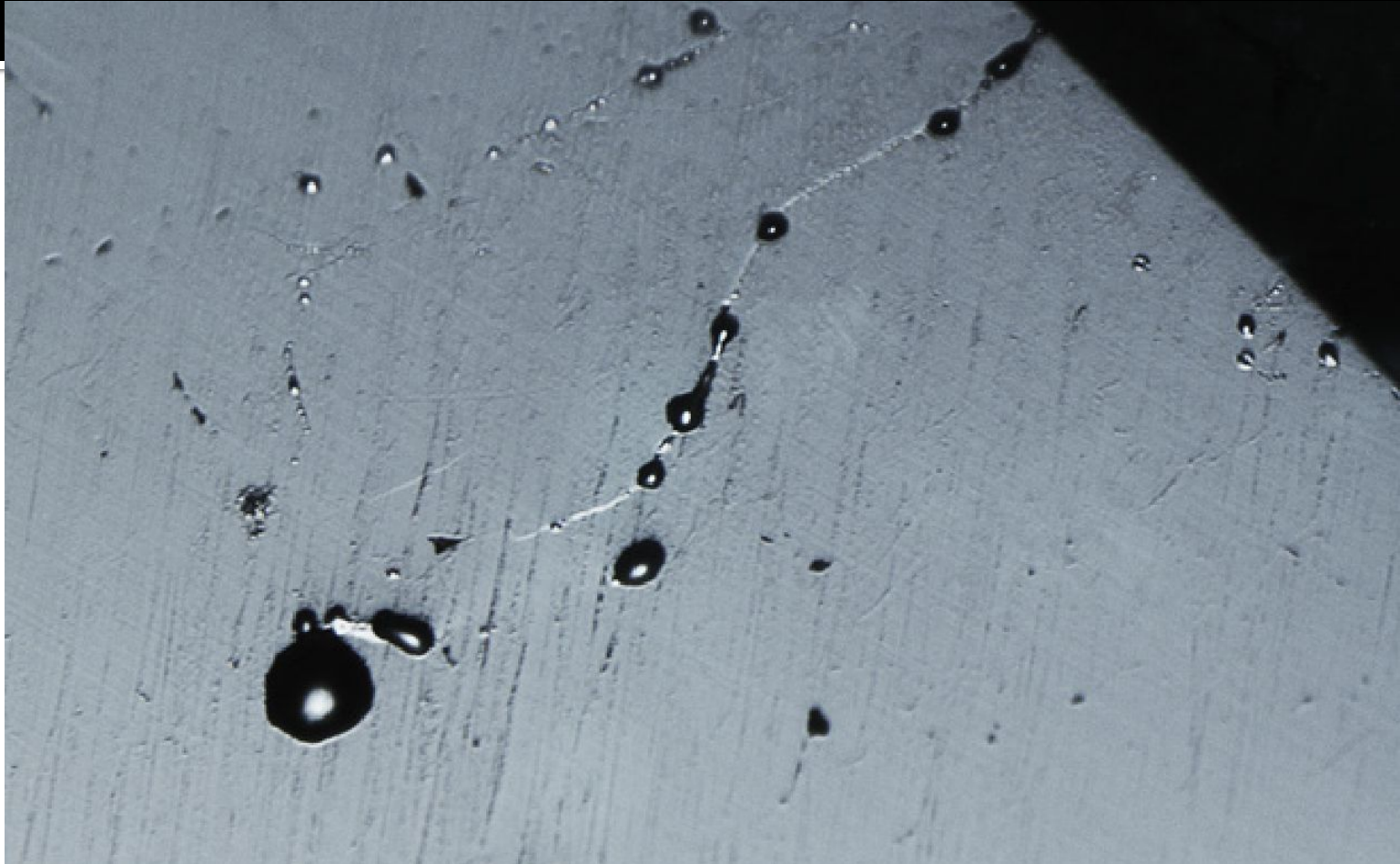
Gentle heating along a surface-reaching fracture causes oil to bead on the surface, proving the emerald is clarity enhanced. Field of view 1.72 mm.
