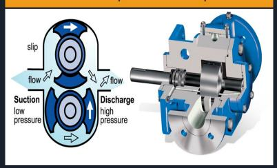
A positive displacement (PD) pump moves a fluid by repeatedly enclosing a fixed volume and moving it mechanically through the system. The pumping action is cyclic and can be driven by pistons, screws, gears, rollers, diaphragms or vanes.
