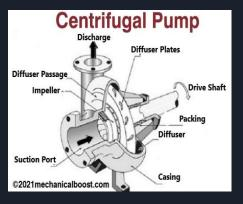
This type of dynamic pump is commonly used in a variety of applications. These types of dynamic pumps are inexpensive to manufacture, robust, and more efficient compared to positive displacement pumps. After the pump has been operated, the fluid pressure increases from the inlet to the outlet of the pump. Changes in the fluid pressure push fluid into the storage tank.
