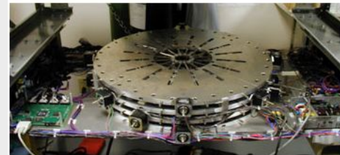
The breast imaging system. Top left: Custom designed four-channel data acquisition module based on DSP and FPGA hardware. Top right: 64 channel EIT system mounted on a mechanical assembly with electrode rods that translate in and out to accommodate different breast sizes. Bottom left: Full EIT assembly on portable cart. Bottom right: EIT system mounted beneath a clinical breast biopsy table.
