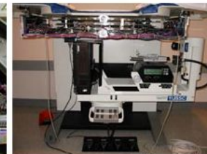
The breast imaging system. Top left: Custom designed four-channel data acquisition module based on DSP and FPGA hardware. Top right: 64 channel EIT system mounted on a mechanical assembly with electrode rods that translate in and out to accommodate different breast sizes. Bottom left: Full EIT assembly on portable cart. Bottom right: EIT system mounted beneath a clinical breast biopsy table.
