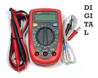
Modern multimeter. Shows more accurate readings in contrast to analog. It has more advanced features (for example, such as "temperature measurement"). The disadvantage is the lack of battery life without a third-party power source.
